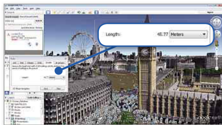
Use Google Earth Pro's 3D ruler to measure heights or calculate the area of 3D surfaces
